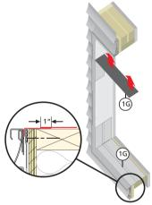
H. **Apply sill flashing tape #1.** (Wood wall construction only). Cut a piece of flashing tape 12" longer than the opening. Apply at the bottom up to the exterior edge of the opening as shown. If the sheathing or water barrier
